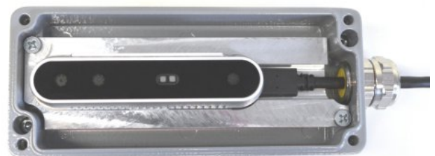
The mount guarantees good heat dissipation
