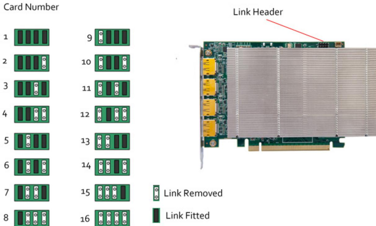
The links control the order in which the display driver uses the ImageDP4 cards. Knowing the order in which the ImageDP4 cards are used is useful when connecting the screens and the outputs from video switches.
