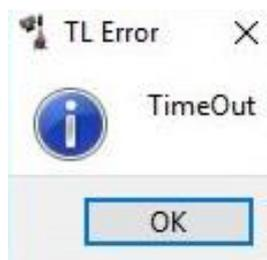
This error appears when the acquisition of one frame needs longer than the **Heartbeat Timeout** is adjust. By default this time is 3000ms. Reduce the Profiles per Frame or reduce the Sensor Frame Interval time for a faster profile acquisition. If the Sensor Frame Interval is already at the lowest possible value reduce your AOI size to acquire faster frames.
