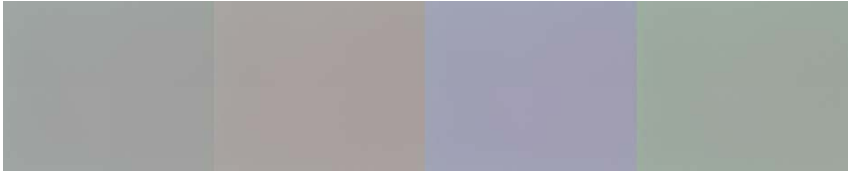
Figure 4. Stitching four images from cameras with the same white balance gains; the scene is a white wall uniformly illuminated with studio lamps (image was slightly altered to make the differences more obvious)
