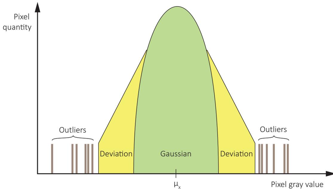
Figure 1: Schematic logarithmic histogram of a camera model
