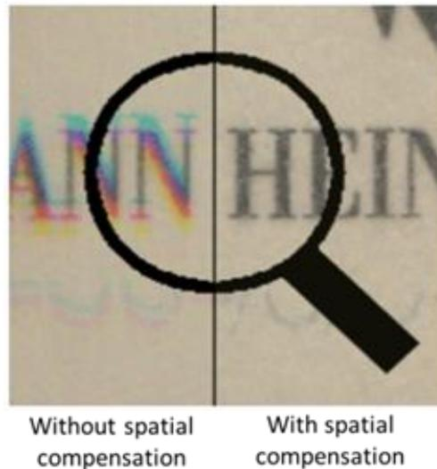
*Fig. 9 - Spatial compensation in trilinear cameras (image from AIA training material)*
