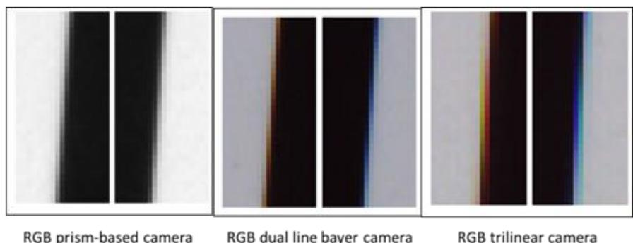
*Fig. 7 - Image quality of a moving printed web using different camera technologies*
