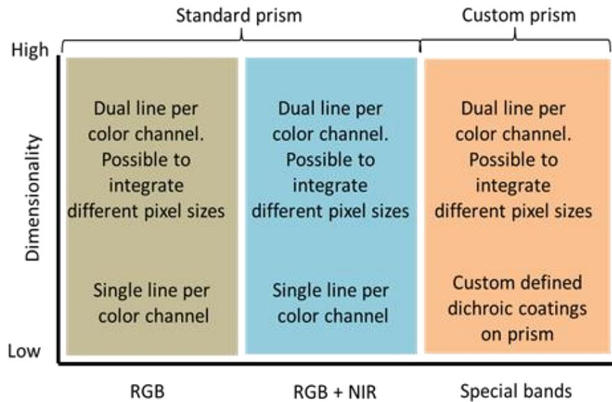
Fig. 3 - Configurations with multi-sensor prism-based line scan cameras
