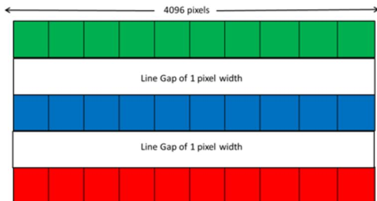
*Fig. 8 - Spatial compensation in trilinear cameras (image from AIA training material)*
