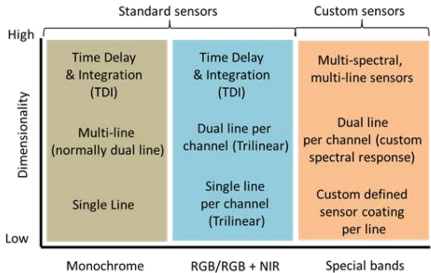
*Fig. 2 - Configurations with single-sensor line scan cameras*
