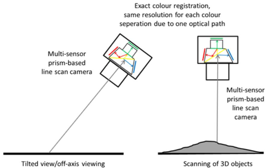
*Fig. 6 - Prism-based line scan cameras in off-axis and 3D object inspection*
