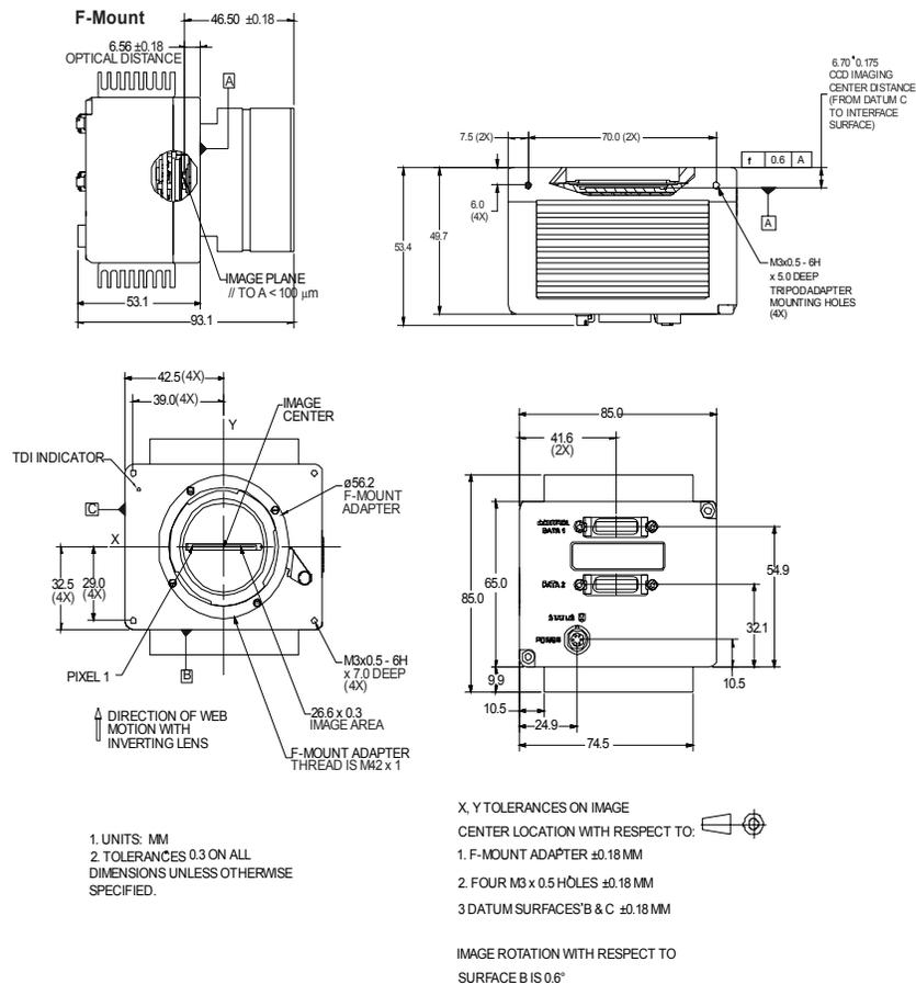
**Figure 13: Direction of Web Movement using an Inverting Lens**
