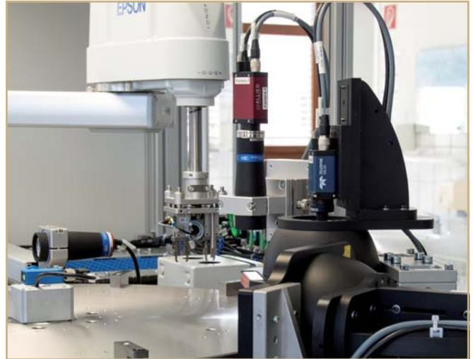
Numerous automation and machine vision systems are integrated in Zorn's inspection system to check shiny metal parts for fuel injection pumps used in the automotive industry.
