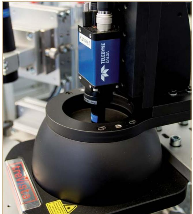
The Trevista imaging system (with a Teledyne DALSA camera) operates with the patented Shape-from-Shading process that determines the three-dimensional form of an object from its distribution of brightness and surface shading.
