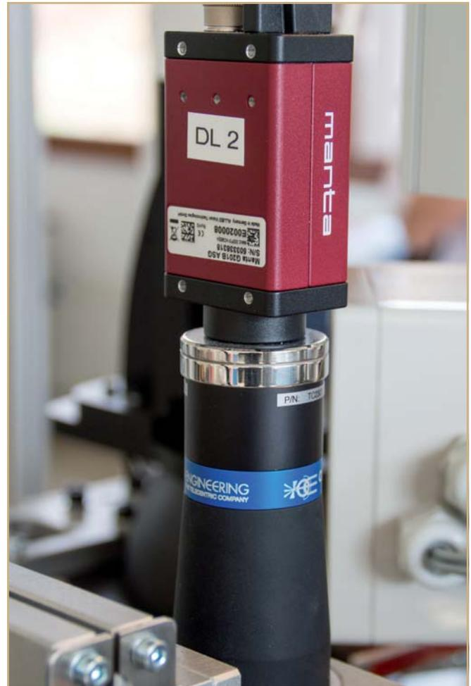
Precise image acquisition thanks to the AVT Manta camera and Opto Engineering's telecentric lens.
