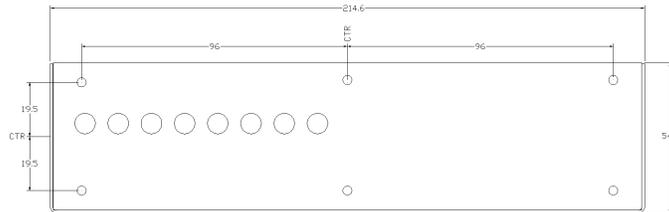
The PP820 enclosure is a fire enclosure as long as the following conditions are met. The unit must be mounted either with the mounting face horizontal or downwards or with the large face of the base horizontal and downwards. All downwards facing holes must have a screw in them.
