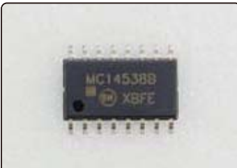
Lead, print, and defect inspection of electronic component package
