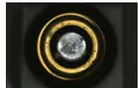
It is possible to evenly illuminate the whole solder, including the cap.
