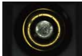
It is difficult to evenly illuminate the whole solder.
