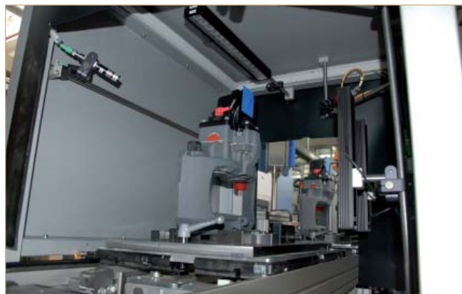
Three cameras, different illumination units and two line lasers are in use in the test cabin.
