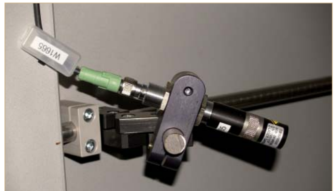
Detailed view of one of the line lasers used. These illumination systems form the basis for the acquisition of characteristics according to the triangulation method.
