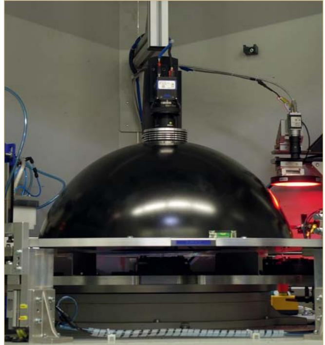
The hybrid components of the steering control are fed to the trevista system and recorded there using the 12 megapixel camera Genie TS by Teledyne DALSA.
