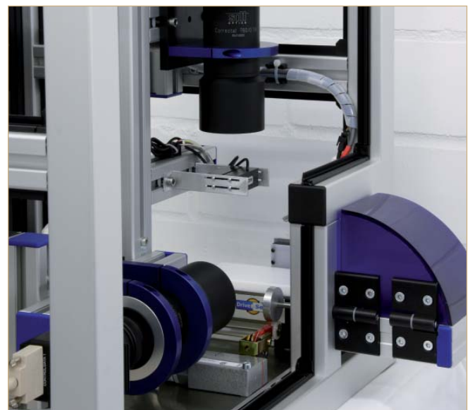
An integrated linear system accelerates the bar to be tested within a few cm and then moves it with constant speed below two line scan cameras.
