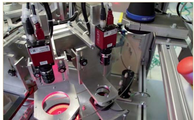
The parts for inspection are transported on a glass ring and pass clockwise through all stations.
