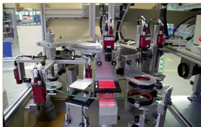
Twelve cameras at six stations ensure reliable detection of faulty parts.
