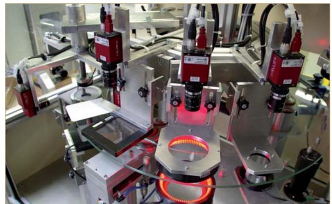
On four of the five stations, the items for inspection are analysed from top to bottom.
