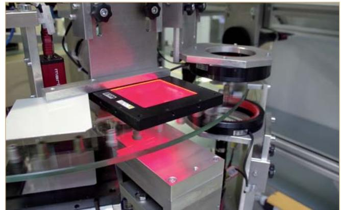
LED illumination in various designs and different directions provide optimal lighting at each station.
