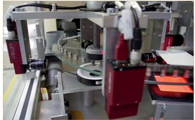
Four cameras at the final inspection station record the screw from all sides. To the right one can see the illumination flash of the penultimate station.
