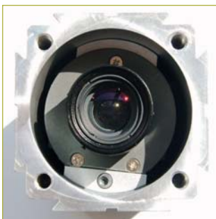
Camera mounting with continuously adjustable position
