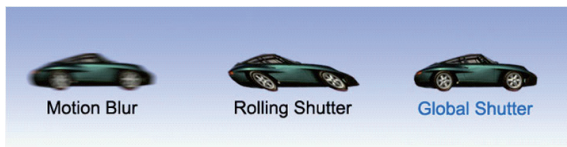
Figure 3: Global shutter, rolling shutter and image distortion
