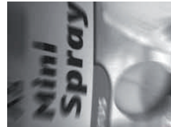
Without tilt adjustment, the object is not homogeneously focused.
