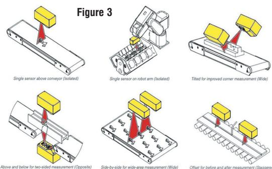
**Figure 3. Single and two camera measurement configurations**
