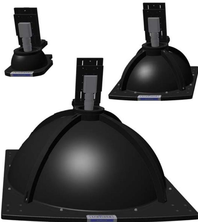
The illumination housings are available in three different sizes to allow components up to 200mm diameter to be measured
