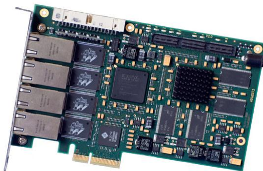
Figure 3 – Silicon Software VQ4-GPoE – a four-channel PoE card with two on-board FPGAs; one to perform acquisition tasks without burdening the PC's CPU, the other to provide user-programmable vision processing.
