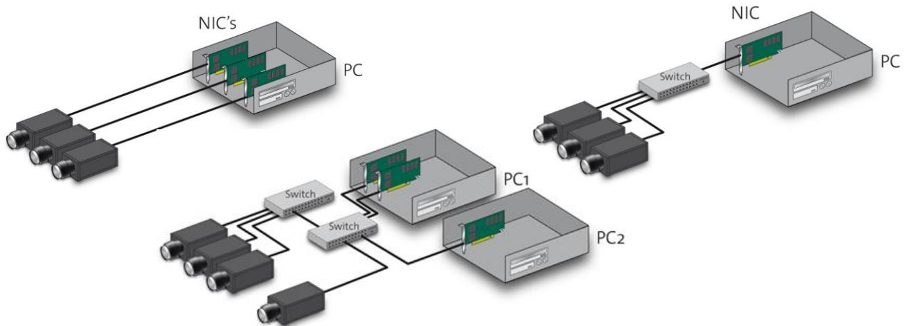
Figure 2 – different network topologies for cameras and PCs. The best arrangement requires consideration of the bandwidth requirements.
