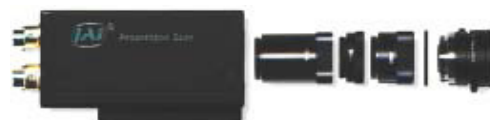
Figure 5 – Extension tubes are placed between the camera and the lens to reduce the minimum operating distance of the lens.
