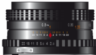
Figure 3 – F-mount lens diagram showing focus adjustment (top ring) and aperture adjustment (bottom ring) with f-stops marked.
